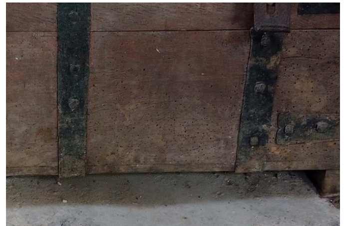
Photo: Historic common furniture beetle damage on a medieval church chest
